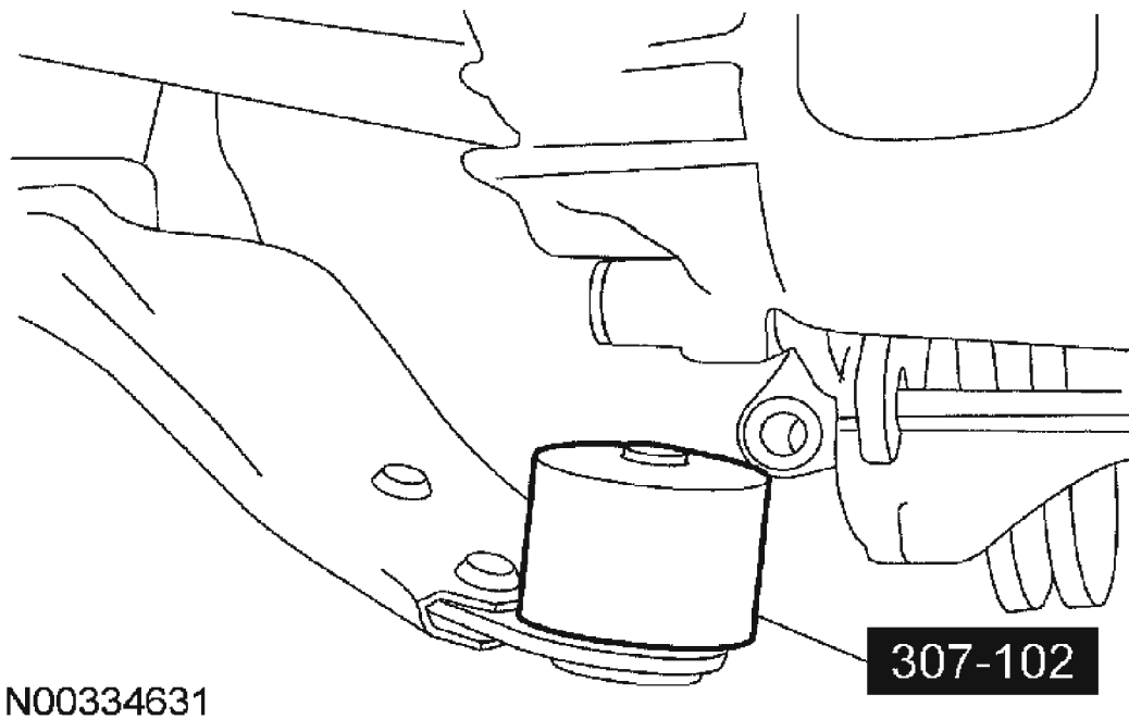
Fig. 17: Install The Special Tool Over The Ball Stud Courtesy of FORD MOTOR CO.
