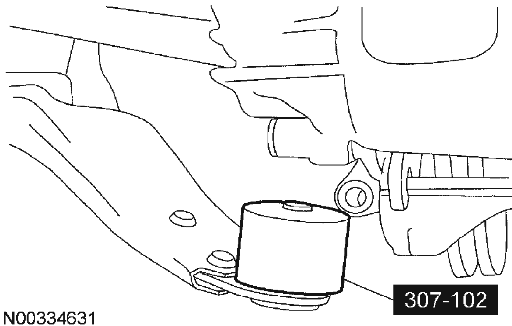
Fig. 6: Installing Special Tool Over Ball Stud Courtesy of FORD MOTOR CO.
